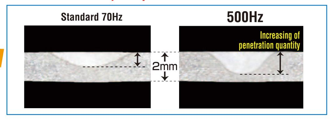
Effect 2. Tack Welding and Starting Speed will be increased triple by Instantaneous Pool Formation
